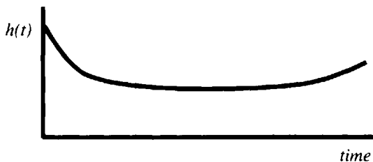
Figure 3.2 A typical bathtub curve for mechanical devices.
